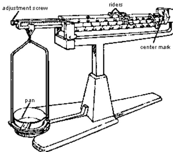
**D.** When the pointer is zeroed, sum up the masses shown on the beams. Remember, significant figures are all figures known with certainty AND ONE GUESS. With our scales, we can read down to the hundredths place for CERTAIN and we can GUESS the thousandths place. Therefore, in this class, ALWAYS record all masses to THREE PLACES PAST THE DECIMAL POINT.
