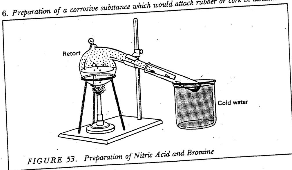
FIGURE 53. Preparation of Nitric Acid and Bromine
