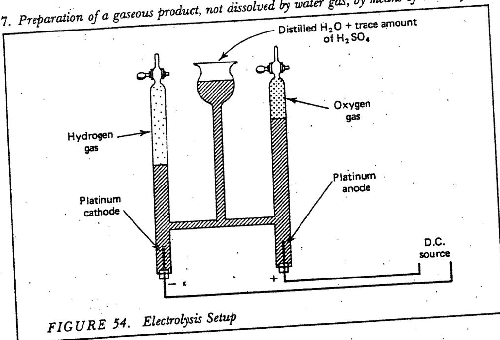
FIGURE 54. Electrolysis Setup
